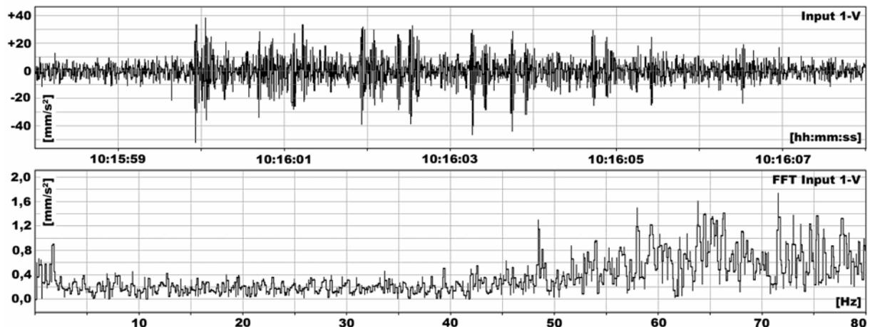
Figure 2: Vertical vibration of pile head excited by a train passing through a tunnel Prague line B (the whole course – up, frequency spectrum – bottom).
