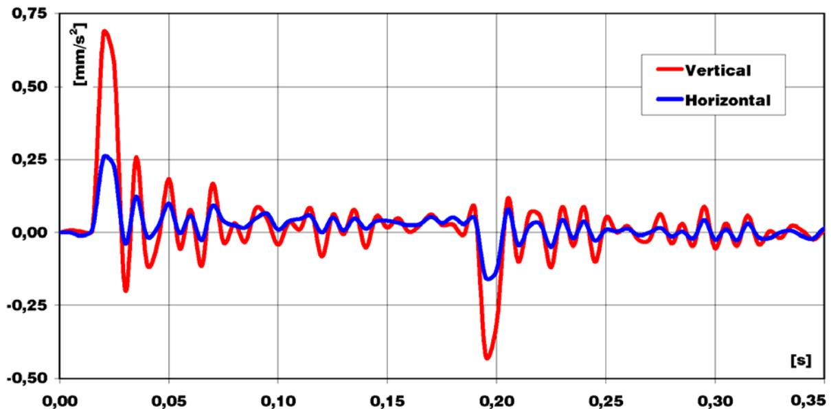
Figure 3: Vibration of pile heads excited by a train passing over the boundary between the under-ground and above-ground bridge part of the tunnel structure.
