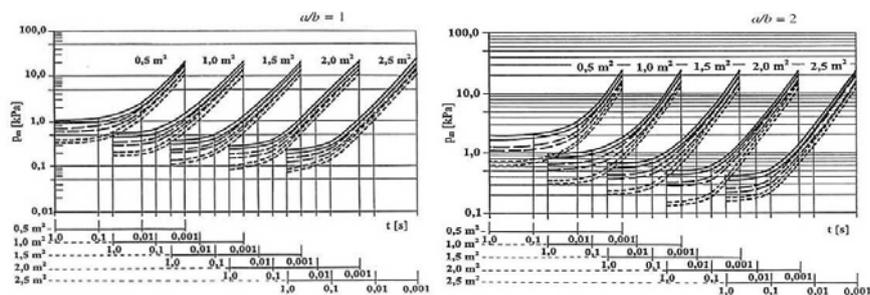
Figure 2: Bunch graph for the computation of window glazing breaking in dependence on overpressure  $p_m$  of the loading impact wave, overpressure duration  $t$ , glazing area  $A$ , glass thickness (3 mm – dotted line, 4 mm – dash-and-dot line, 5 mm – solid line) and window glass age (pairs of lines of the same type define new glass and ten-year old glass); ratio of window glass dimensions a)  $a/b = 1$ , b)  $a/b = 2$
