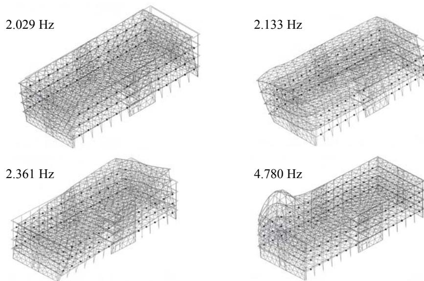
Figure 3: The lowest natural frequency of building vibrations
