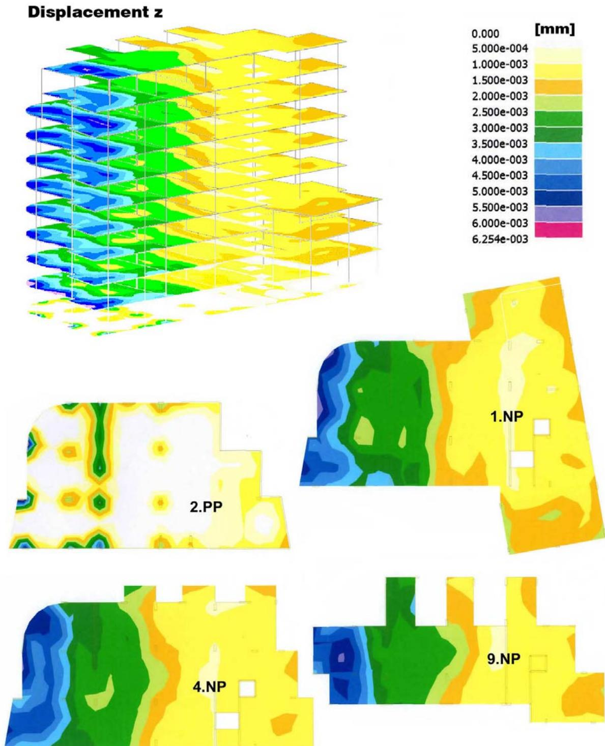
Figure 7: Maximum vertical displacements of selected storeys
