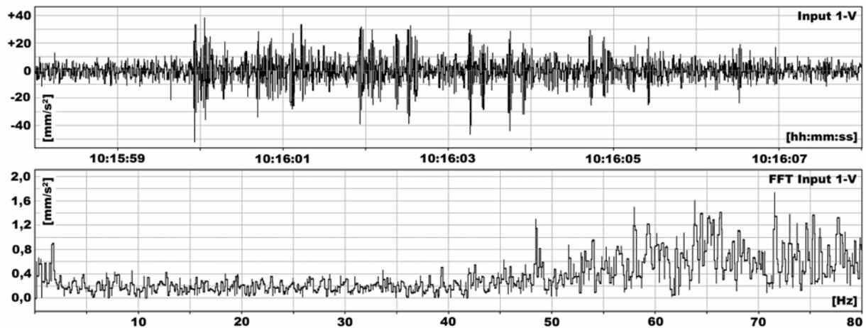
Figure 2: Vertical vibration of pile head excited by a train passing through a tunnel Prague line B (the whole course – up, frequency spectrum – bottom).
