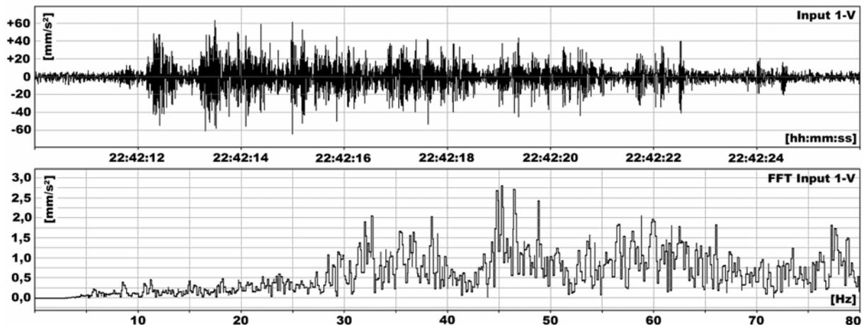
Figure 1: Vertical vibration of pile head excited by a train passing through a tunnel Prague line C (the whole course – up, frequency spectrum – bottom).
