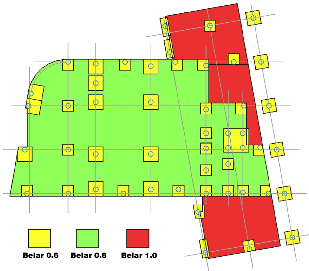
Figure 5: Design of rubber distribution (of various rubber types BELAR).
