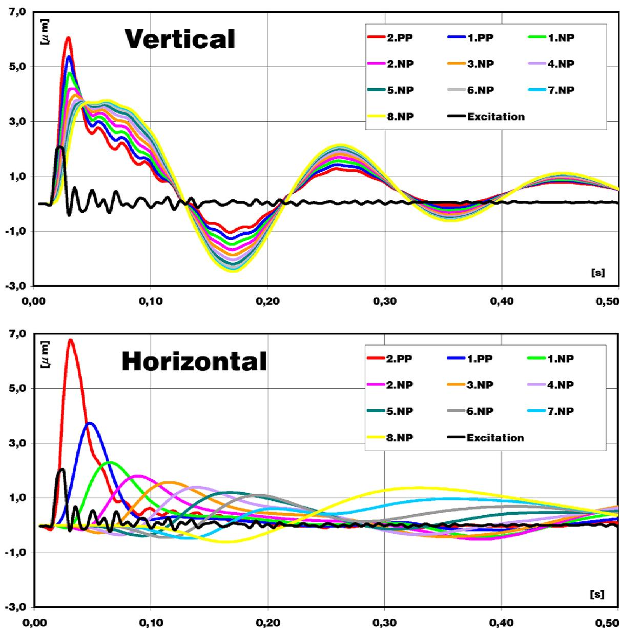
Figure 8: Prediction of vibrations at selected points (located on the structure side near the underground) in storeys as compared with the normalized excitation history in the vertical (up) and horizontal (bottom) direction.
