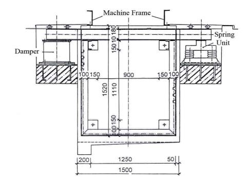
Fig. 2. Cross section of machine foundation.
