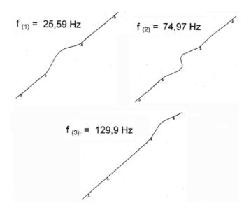
Fig. 5. The first three natural modes of rotor axis.
